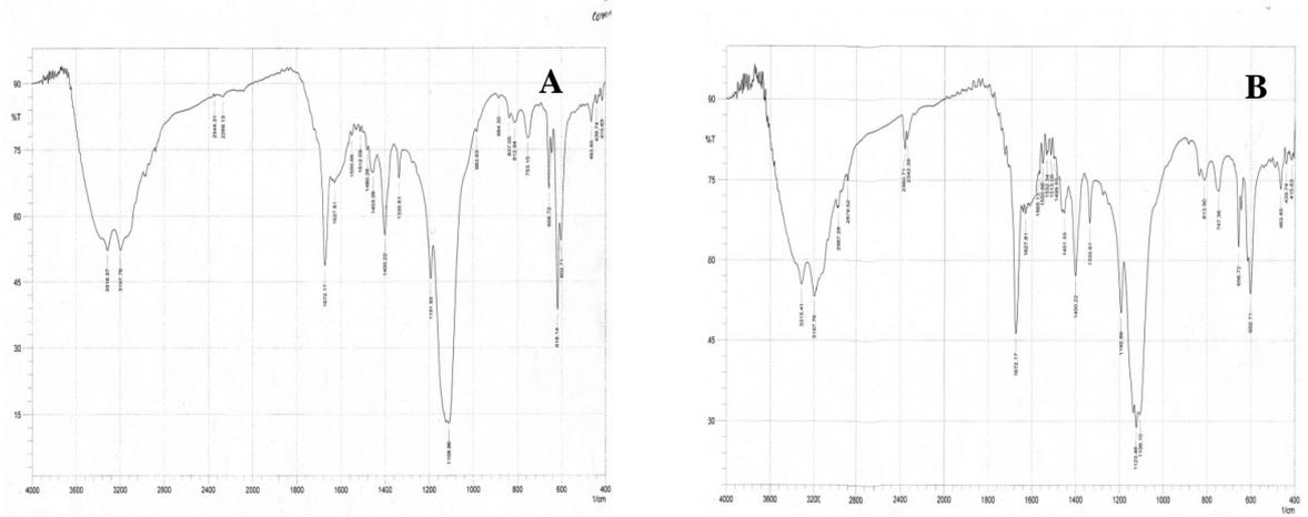
Figure 6. FT-IR spectra of Congo Red before and after adsorption on EOBC
