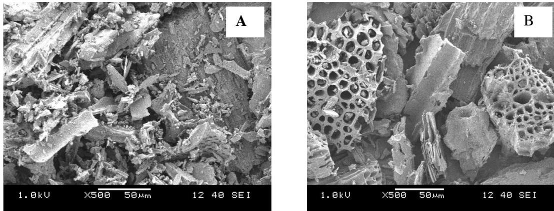
Figure 7. SEM images of OSC before (A) and after (B) adsorption of CR
