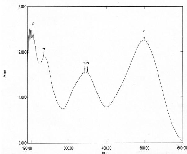
Figure 2 - UV- Spectrum of Congo red dye
