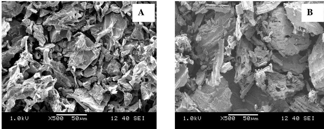
Figure 8. SEM images of EOBC before (A) and after (B) adsorption of CR
