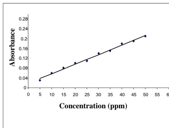
Figure 3. Calibration plot for Congo red dye
