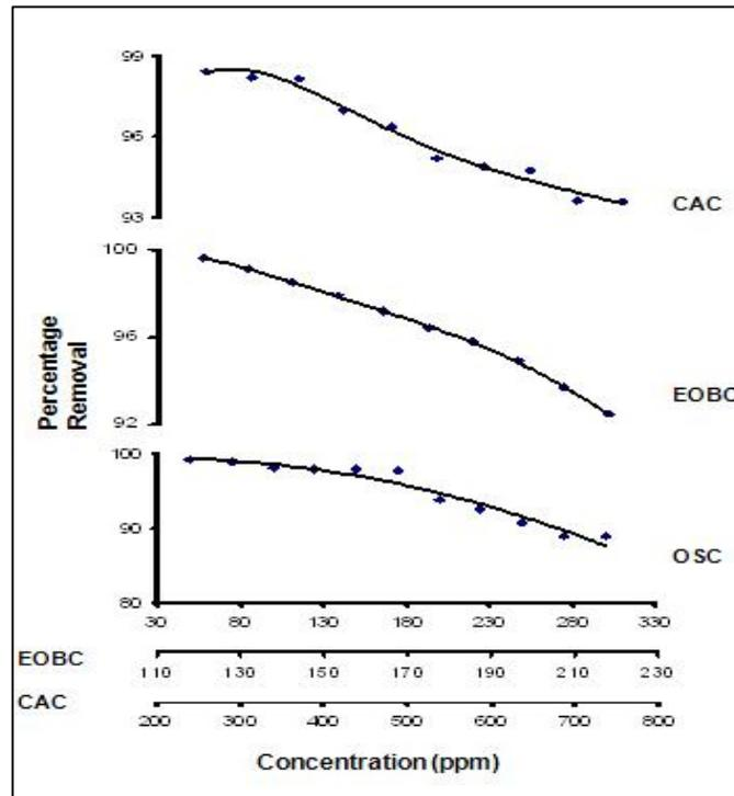
Figure 4. Effect of initial concentration on the extent removal of Congo red dye
